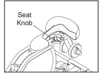
the knob. To determine if the seat is properly adjusted, sit on the seat and pull the handlebar as close as possible to your stomach. Your legs should be almost straight, but your knees should not be locked.
